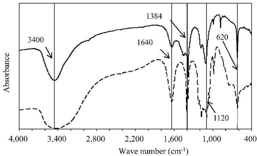
Fig. 7. FT-IR analysis of raw (solid) and treated (dotted) LC.
