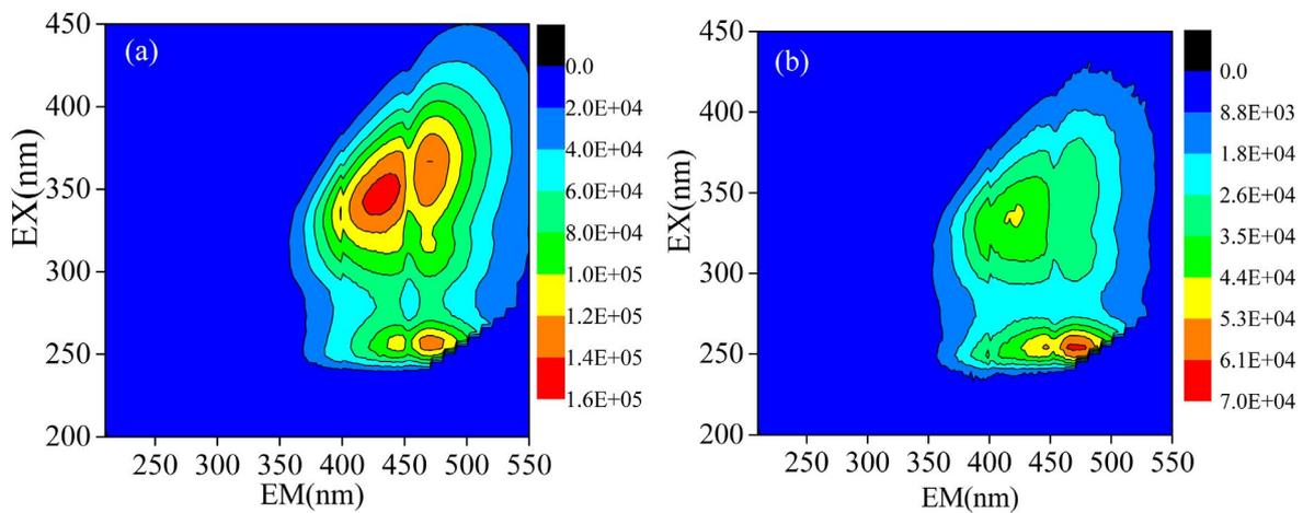
Fig. 8. EEM spectrum of raw LC (a) and coagulation effluent (b).
