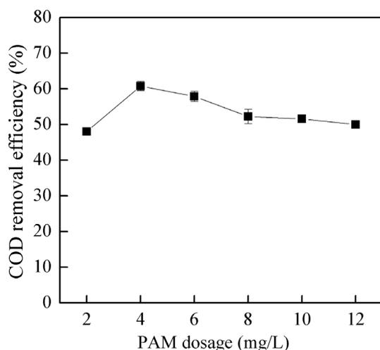
Fig. 3. Effect of the dosage of PAM on the COD removal efficiencies.
