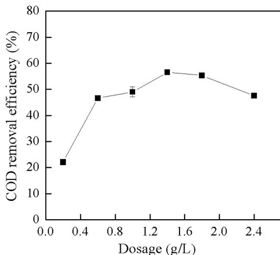
Fig. 2. Effect of the dosage of  $\text{FeCl}_3$  on the COD removal efficiencies.
