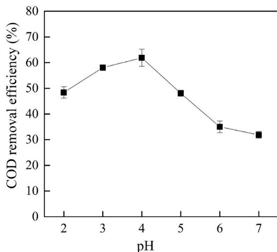
Fig. 1. Effect of pH on the COD removal efficiencies.
