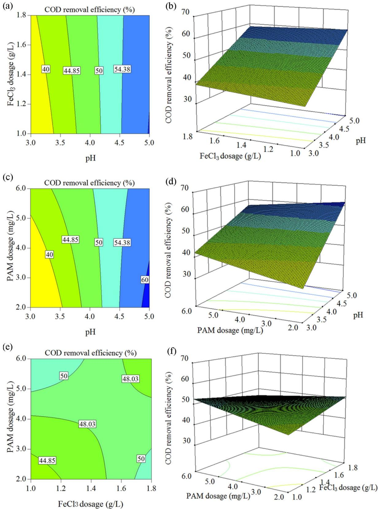
Fig. 4. Contour (a, c, e) and response surface (b, d, f) plots of the COD removal efficiency as a function of pH and the FeCl<sub>3</sub> dosage at a fixed PAM dosage (4 mg/L); pH and PAM dosage at a fixed FeCl<sub>3</sub> dosage (1.4 g/L); and FeCl<sub>3</sub> and PAM dosage at a fixed pH (4), respectively.
